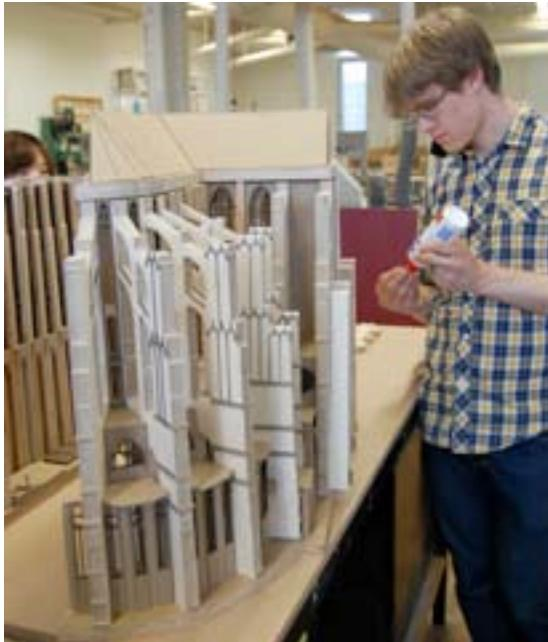
Figure 7: Assembly of Beauvais cathedral buttresses from laser-cut materials by Adam Simonar. (Source: Amr elBahrawy).
