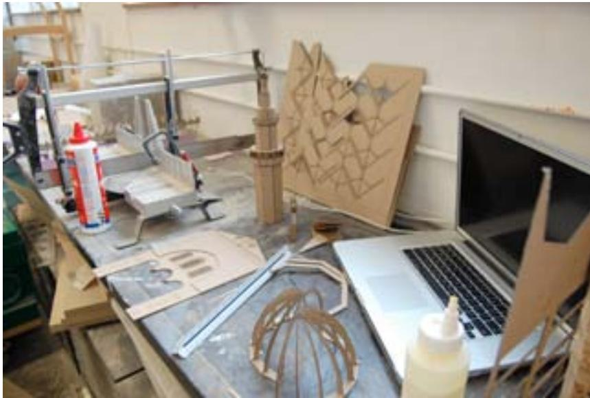
Figure 1: CAD work, Laser-cut panels prepared and assembly of elements in Great mosque of Damascus model (Source: Amr elBahrawy)
