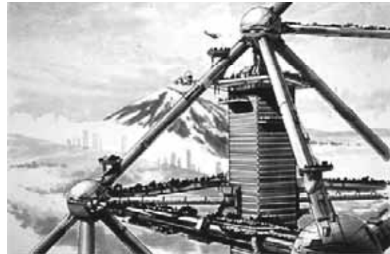
Figure 9: Skyscrapers Hung from Critical Truss Joints which also Function as Transportation Hubs in the Mega City Pyramid (Dante Bini, www.binisystems.com ).
