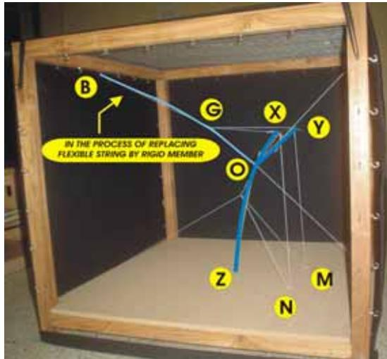
Figure 5 : The forked end X-Y was further stabilized by tying the free ends, hence restricting the splitting up of elements and forming an inverted triangular prism, dematerialized to expose the wireframe GOXY. An additional bending member BO, to represent the cantilevered roof line was introduced along with the string with an intension to free end B from the jig..
