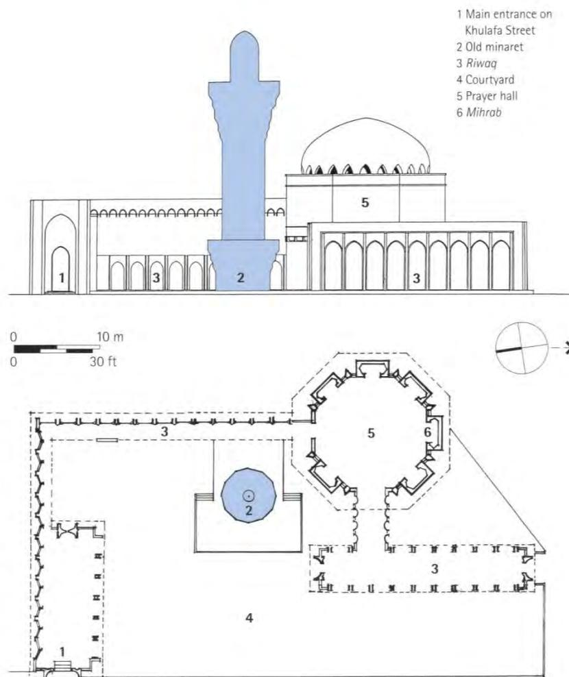
Figure 4A. Plan and elevation of the redesigned mosque with the remaining historic minaret shown in blue.
