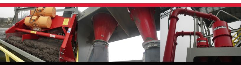
A blend gate on the discharge chute allows the customer to determine how much fine material they want in their final product by allowing a portion of the fines to be mixed back into the coarse sand stream. Spray bars on the Dewatering Screen offer the ability to provide a final rinse of the material before it is discharged. This allows some of the fine material to make its way down through the screen, into the sump and onto the fine side of the screen where it belongs.
