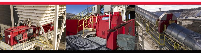
Sampling System consisting of a primary Cross Belt Sampler, Sample Hammermill and secondary Falling Stream Sampler.
