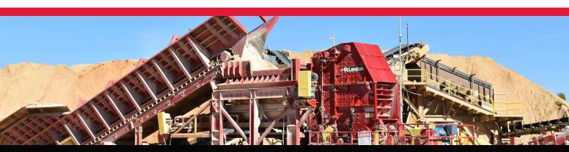
To feed the MaxCap and round out the portable primary plant, Anderson Columbia installed a unique configuration of an Apron Feeder, referred to as a Texas-style apron, and a Wobbler Feeder. The Apron Feeder accepts bucketloads of quarry shot material and conveys it to a Wobbler Feeder. The Wobbler Feeder is able to scalp out some of the clay before it enters the MaxCap Impact Crusher.
