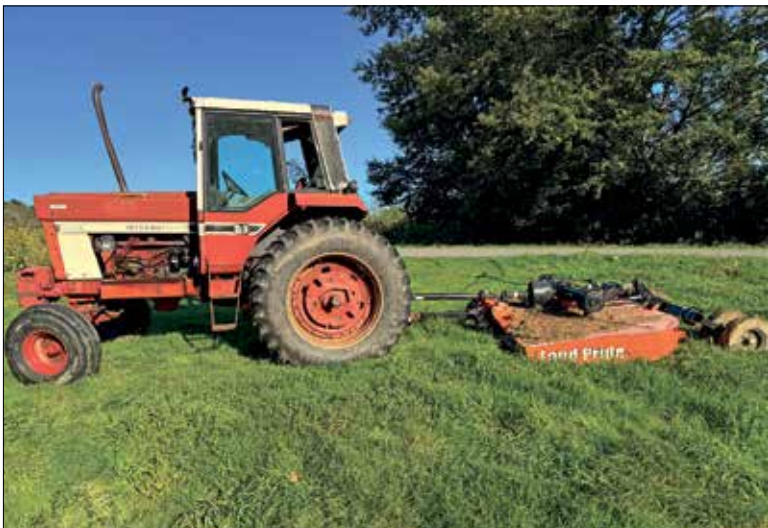
The author’s 10-foot brush hog, which attaches to the drawbar and is raised and lowered hydraulically.
