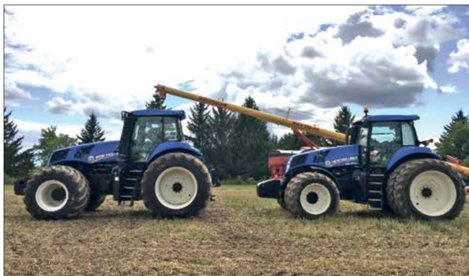
A tractor equipped with high-flex sidewall tires (left), capable of operating in fields at low tire pressures, compared to a tractor with standard high pressure tires (right). Kitty O'Neil / Cornell Cooperative Extension
