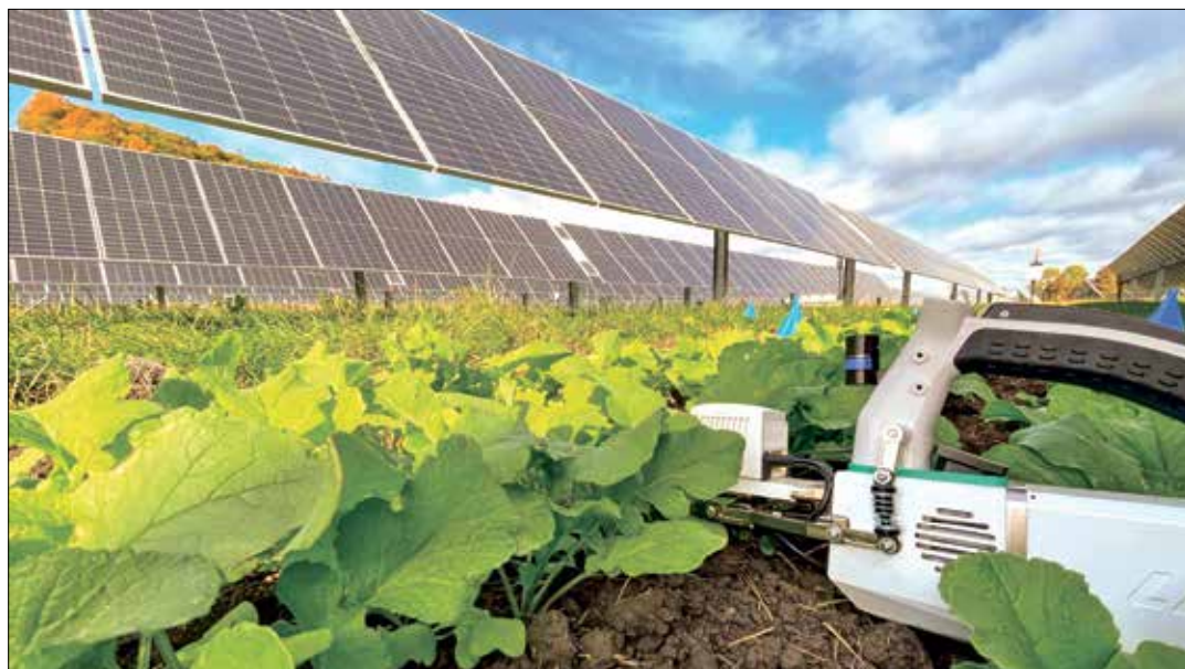
An infrared gas analyzer assesses photosynthetic light response in radish plants grown on a solar farm near Albany, NY.
