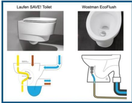
Special “split bowl” UD toilets are designed to collect urine in the front of the bowl and are now being designed and sold by major manufacturers. This allows separation and requires the user to sit. Urine flows through piping into a holding tank, which is pumped periodically. The urine can then be treated and processed as fertilizer.
