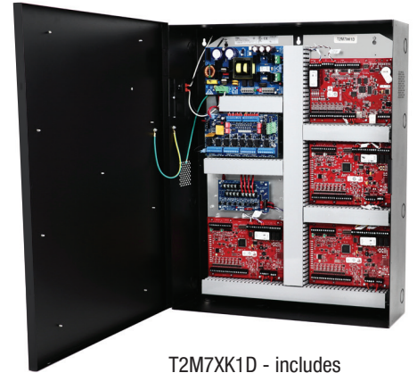
T2M7XK1D - includes eFlow104NB, ACMS8CB, VR6, PDS8CB, wire harnesses and finger duct
