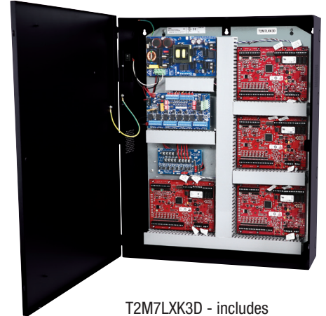
T2M7LXK3D - includes AL1024ULXB2, ACMS8CB, VR6, PDS8CB, wire harnesses and finger duct
