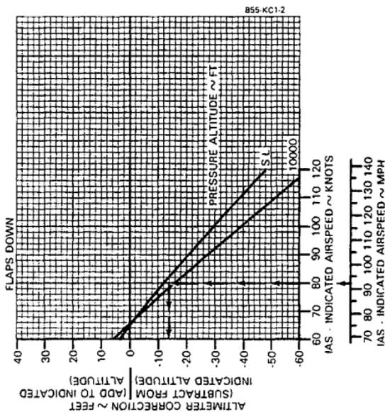
AIRSPEED CALIBRATION - ALTERNATE SYSTEM
