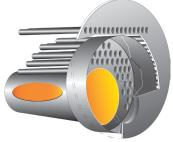
Large Wet-Back combustion chamber with low heat release for complete comubstion **STEAM**Pressures to 300 PSI.
