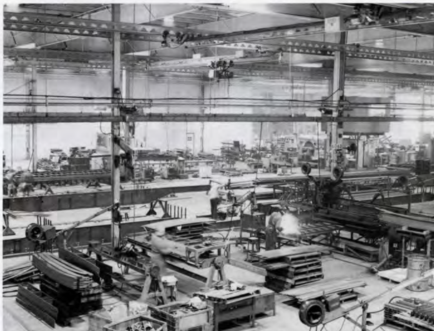
The background area of photo shows the light intensity created by the high pressure sodium lights. In foreground, mercury vapor light bulbs light the work area
