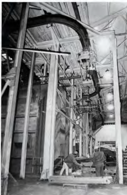
The motorail shot blast machine was custom designed for LUFKIN to handle large castings. The inside cabinet has a height of 20 ft. which allows cranks up to 18 ft. to be cleaned
