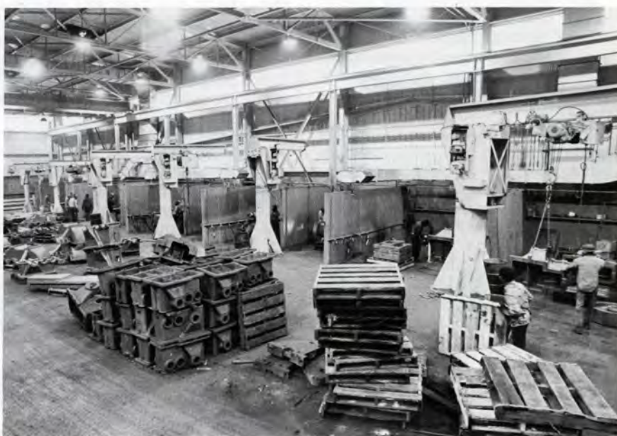
The individual booths of the cleaning room are equipped with a chipping gun, a grinder, and a jib crane
