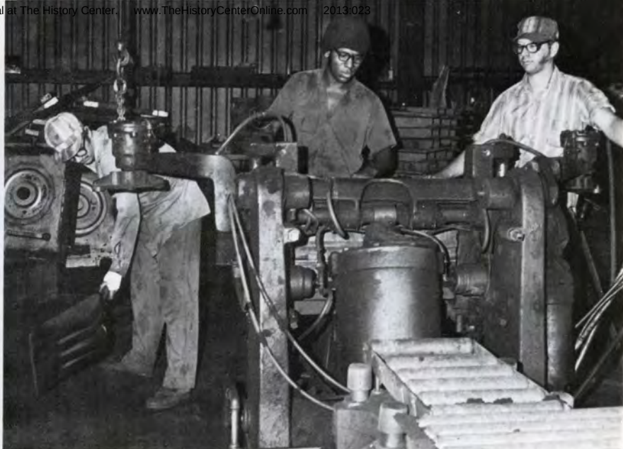
Walter Oder, left, Curtis Dupree, center, Donnie Dudley ram the drag half of a mold to pack the sand
