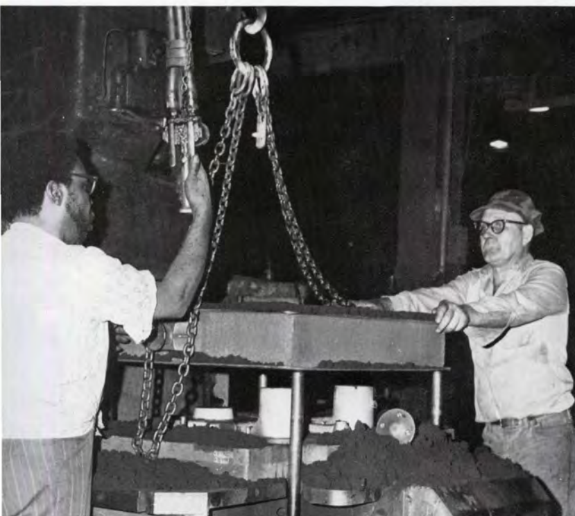
Harold Hicks sets mulling time to mix molding sand. Usually, every three minutes, a muller mixes about 4,500 lbs. of sand
