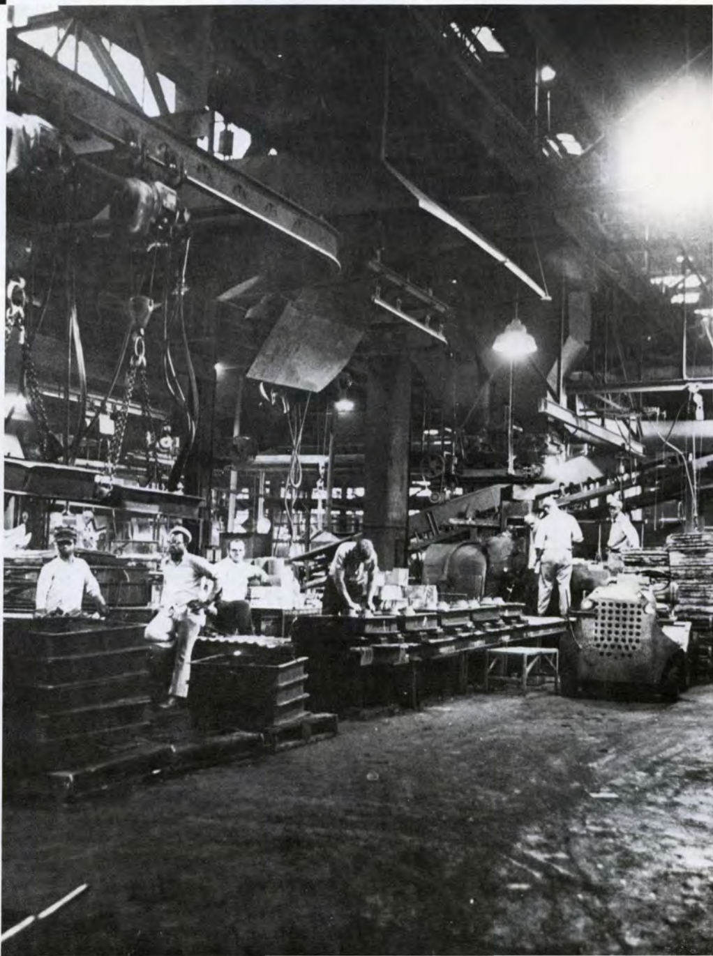
Walter Oder, left, Curtis Dupree, center, Donnie Dudley ram the drag half of a mold to pack the sand
