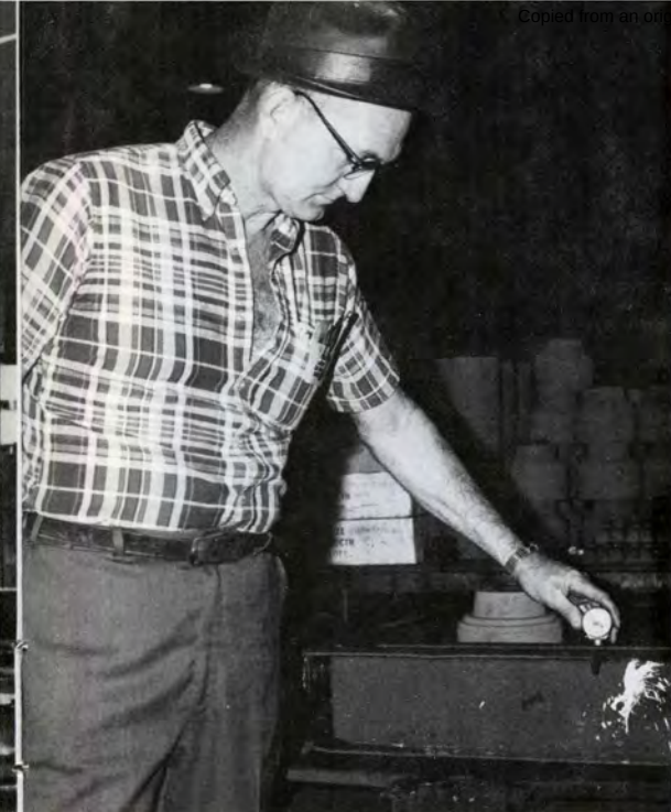
James Jones, new foreman of the counterweight foundry, checks green strength (hardness) of sand. A green strength of 80 degrees indicates the sand is sufficiently hard for the pouring of metal
