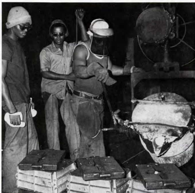
James Dairden, left, Joe Grogan, and John Norman are pouring metal into "squeezer" molds
