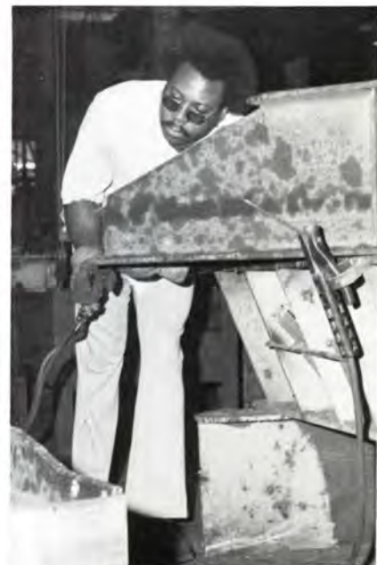
In order to fit a plate on an equalizer, setup man Willie Washington burns a point off the end
