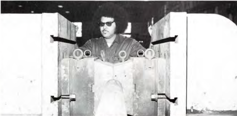
Set up man Aron Garner operates a bulldozer which bends pipe for side members and head plates of pumping units
