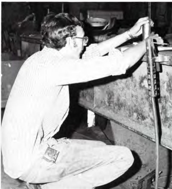
Roger "Snake" Moore places a shaft on the foot plate to set up a brake trunnion
