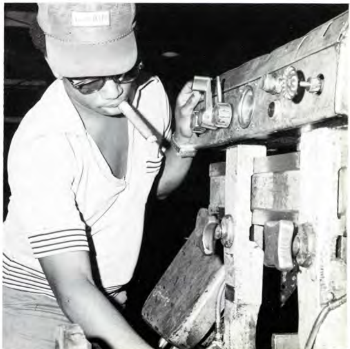
In order to fit a plate on an equalizer, setup man Willie Washington burns a point off the end
