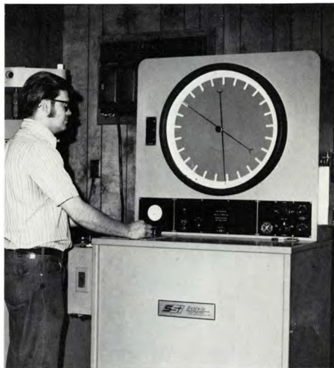
DON demonstrates the operation of the new strength testing machine, which gets plenty of use by both the Industrial Engineering department and metallurgical lab
