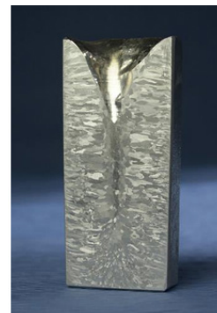
Pure aluminum with columnar grains
