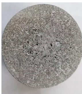
Figure 2. Comparison of aluminium macrostructure. Note the more homogeneous structure in the NUCLEANT-treated sample.
