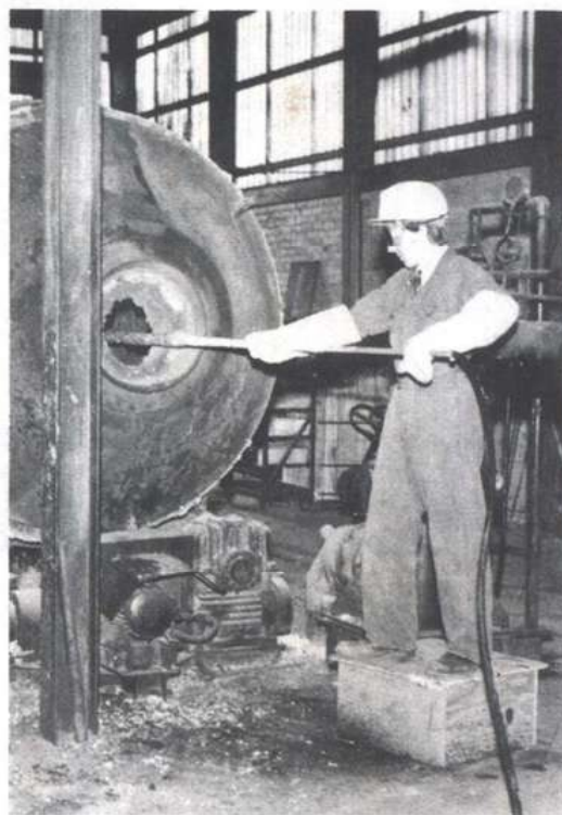
Fig.15. Carburation in a rotary furnace by graphite injection.
