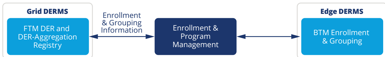
Figure 6. Utility DER Program Enrollment Process and DERMS
