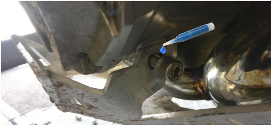
With back of skid plate loosely attached align front of skid plate with front mounts at the bottom of the engine. Using (2) M10 x x25 socket head cap bolts included with the brackets, apply thread locker, and (2) M10 washers (one for each side), do not fully tighten.
