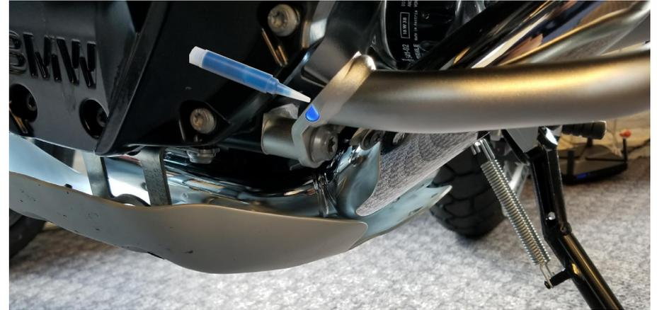
**BMW Crash Bars:** The AltRider skid plate goes in underneath the spacer and crash bar shown here. Use BMW bolt and spacer when attaching the AltRider skid plate. Apply thread locker.
