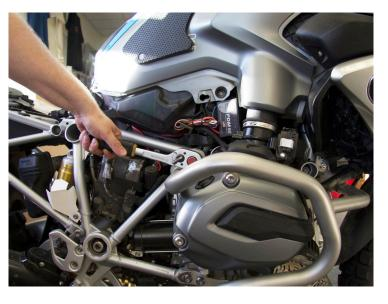
Using two 18 mm sockets, tighten the M12 engine bolt and then torque to 85 nm.
