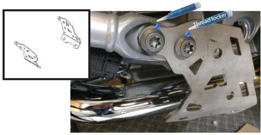
2 Starting with the right side install the brackets with (2) OEM M10 Torx bolts and apply thread locker. Get all fasteners started but do not tighten yet. Repeat on the left side. See diagram above for reference. TIP: take your time getting the frame aligned with holes in engine mounts. Note: If the holes are not aligned have a helper try lifting the rear of the bike slightly to help.
