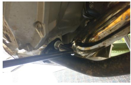
7 Torque the M10 bolts in step 6 to 38nm. Torque M8 bolts in step 5 to 19nm.
