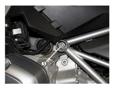
With bike on center stand, remove OEM engine bolt using 18mm socket and T55 driver. Use a 1/4" extension to push the bolt out far enough that you can grab it and remove by hand. Save the nut for step 4.
