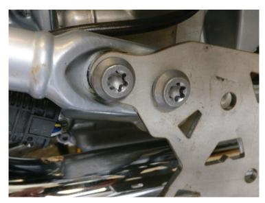
Return to bracket bolts listed in step #2 and torque the M10's to 55nm.
