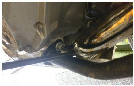
Install the M10 x 25mm bolt and washer, found in the bracket kit, to the front lower mount position at the bottom of the engine on each side. Insert a spacer between the flange and mounting location if not using AltRider Skid Plate. Use thread locker. Do not fully tighten yet.
