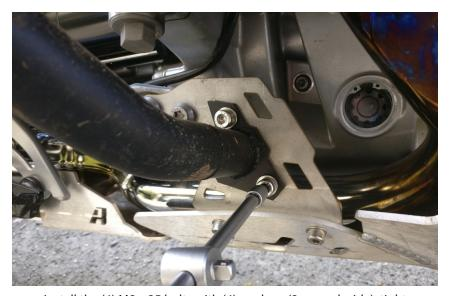
Install the (4) M8 x 25 bolts with (4) washers (2 on each side), tighten with (4) M8 lock nuts. Torque to 38nm
