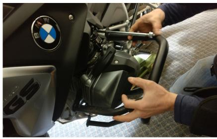
Insert nylon paint protection disc (8) between the crashbar flange and frame boss while inserting the through bolt. Starting with the left side, partially insert engine through bolt into bars as shown above. Feed engine through bolt all the way in, allowing the bars to hang. On the right side insert right side crash bars and attach OEM nut from step 3, apply thread locker.
