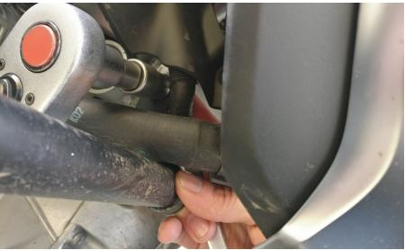
Install the (1) M8 bolt, (2)washers, and (1)lock nut to the top front mount on each side using an M6 driver and 13mm wrench.
