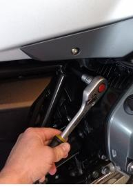
① Use 18mm socket and T55 torx to remove the engine through bolt. You will need to save the OEM Nut, but you will not reinstall this bolt.
