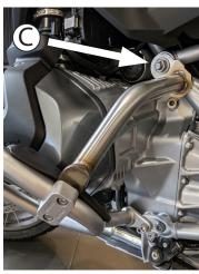
(A) Insert AltRider through bolt through the right hand reinforcement bar, ensuring (3) the (B) mylar washer is between the bar and frame.
