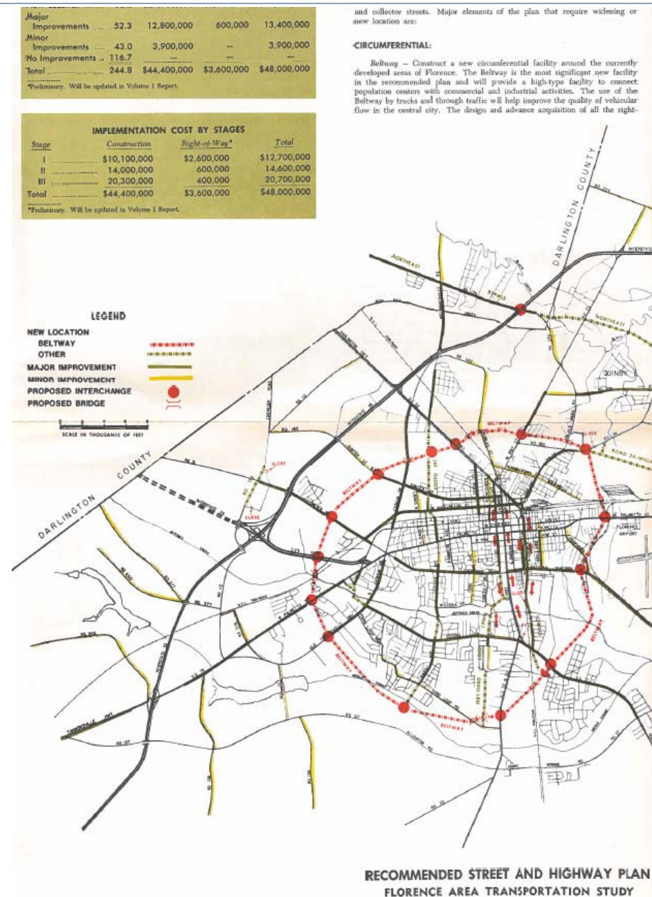
Figure 4 - A Recommended Street & Highway Plan map from a South Carolina State Highway Department published plan of the same name in December 1973 with a horizon plan year of 1995 for the Florence Area Transportation Study. Source: SCDOT
