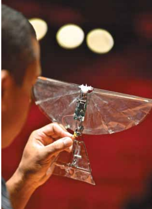
A researcher from the Biomimetic Millisystems Lab from the University of California Berkeley with his flying H2Bird robot, at the Drones and Aerial Robotics Conference (DARC), held at New York University on October 11, 2013.
