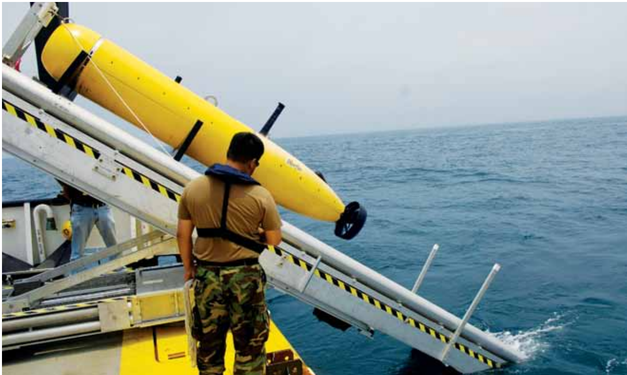
Chief Aerographer's Mate Trung Freed, from Naval Mine and Anti-Submarine Warfare Command, Corpus Christi, Texas, monitors the deployment of a Bluefin Autonomous Underwater Vehicle (AUV) during a day of at-sea testing being conducted as part of AUV Fest 2007, sponsored by the Office of Naval Research, and hosted by the Naval Surface Warfare Center Panama City.
