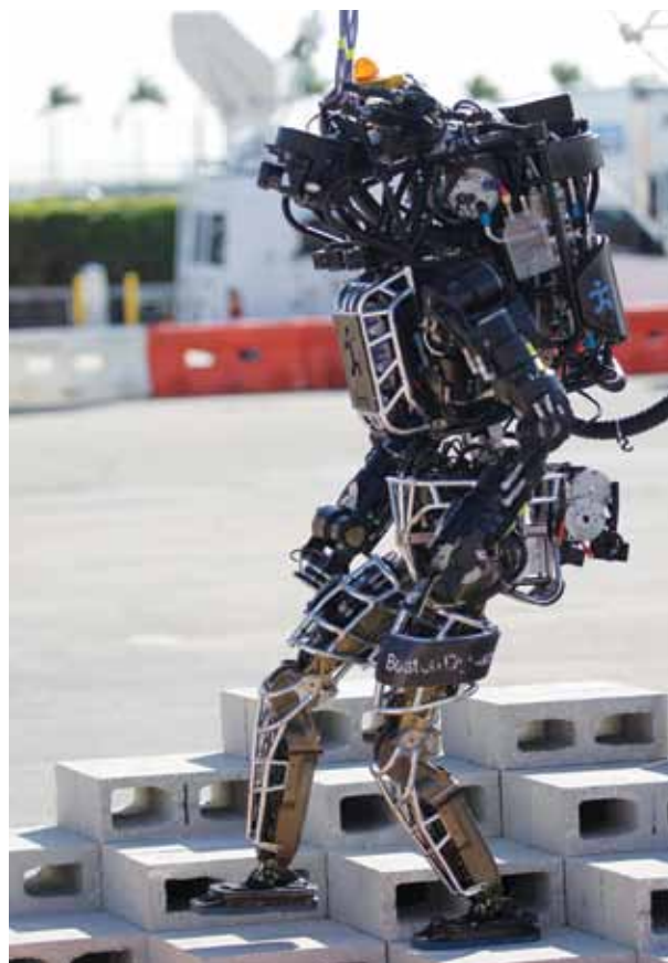
Boston Dynamics' Atlas, a high-mobility, humanoid robot designed to negotiate rough terrain, takes on an irregular surface in this terrain negotiation exercise in Homestead, Florida in December 2013.
