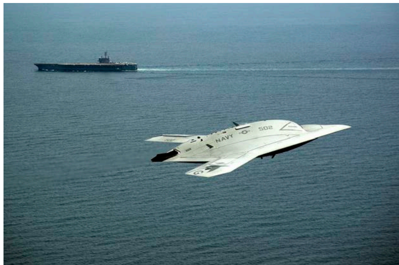
The X-47B (pictured) represents the Department of Defense’s effort to produce a prototype that incorporates stealth, range, and significant internal ordnance capacity. (U.S. Navy)
