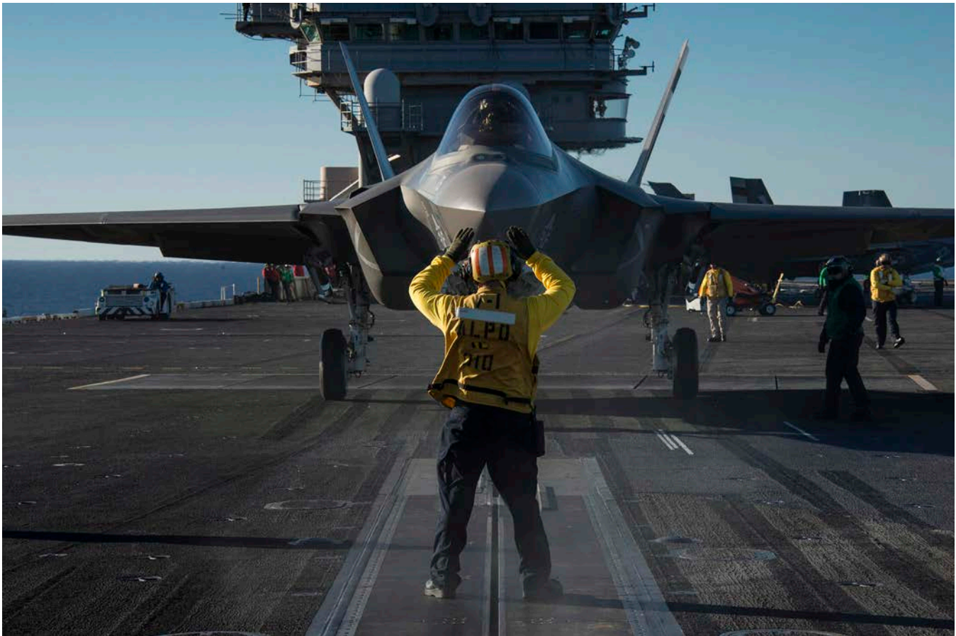
At present the F-35C (pictured) is reported to have an unrefueled combat radius of approximately 625 nautical miles, far short of the F-14 and A-6 aircraft that preceded it on the flight deck. (U.S. Navy)
