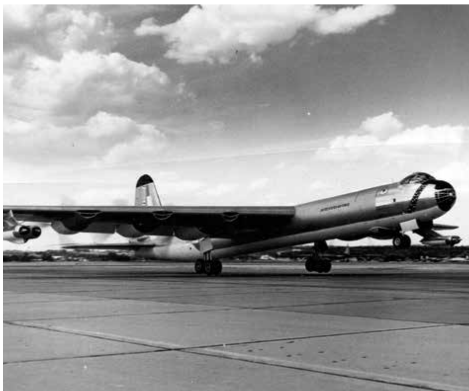
The B-36 was not actually built until 1946, and with the addition of two more jet engines mounted under each wing, its range reached 6,800 miles at a speed of 391 mph, easily outpacing the B-50 by 2,000 miles and over 100 mph. (U.S. Air Force/Flickr)
