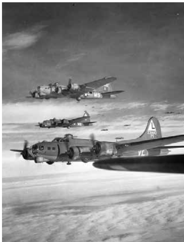
The B-17’s sleek aerodynamic design, four engines, and 103-foot wingspan helped provide it with superior performance that made it America’s front-line bomber. (Air Force/Flickr)
