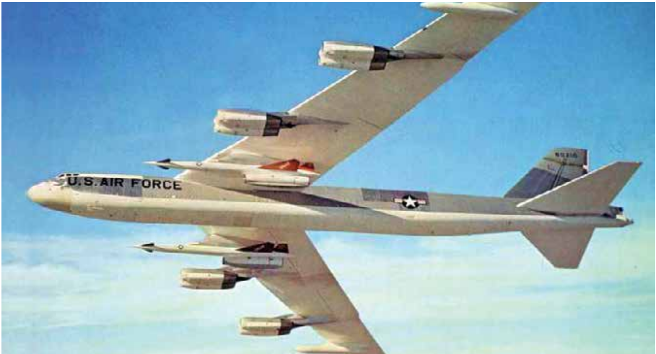
The B-52 could carry two Hound Dog missiles, one under each wing, and use them to clear out concentrated SAMs and AAA sites along its flight path, allowing the B-52 to deliver gravity weapons on its primary targets. (U.S. Air Force/Flickr)
