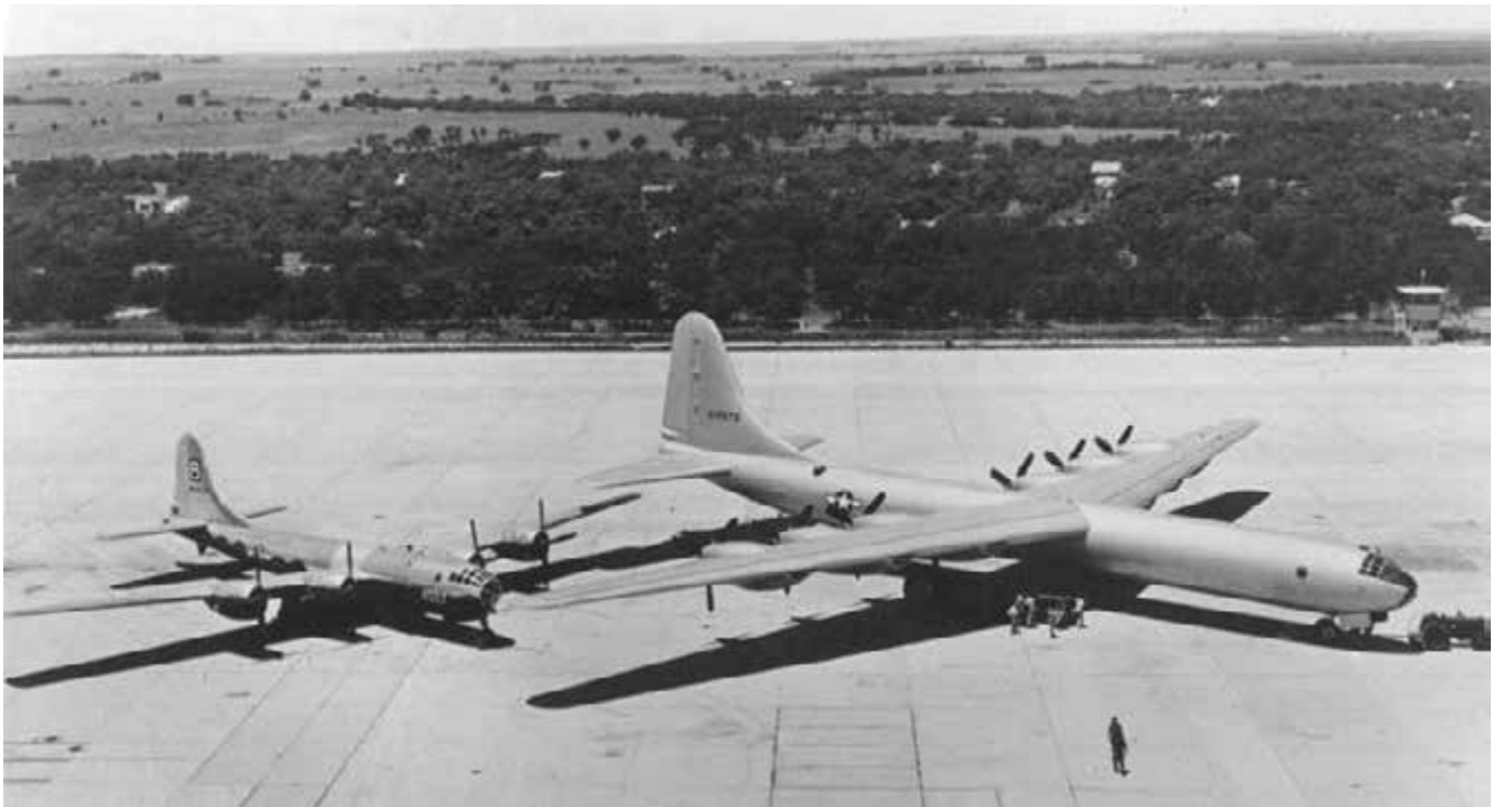
The B-36 was designed to carry a huge bomb load from the eastern shores of the United States to Europe and return to its original point of departure. Everything about this bomber was big. It was nearly twice the size in both wingspan and aircraft weight as a B-29. (U.S. Air Force/Flickr)
