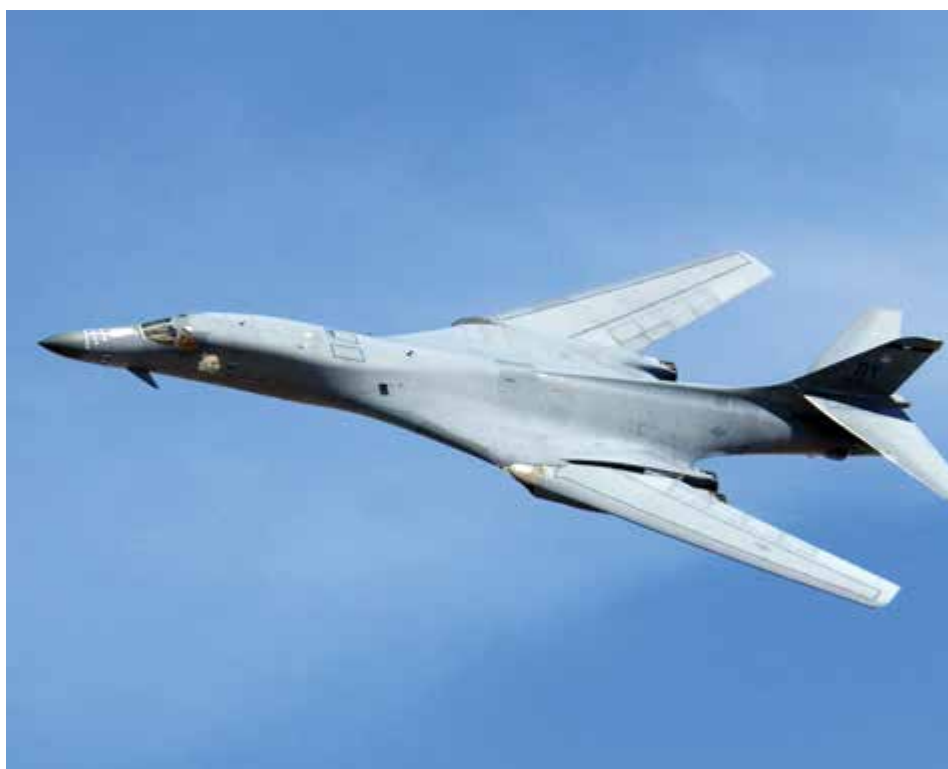
To avoid radar and surface-to-air missile batteries while approaching enemy territory, the B-1 would descend to ground level, sweep the wings back to 65 to 67.5 degrees, and accelerate to ingress enemy territory below the radar horizon, speeding toward the target at supersonic speed. (U.S. Air Force/Flickr)
