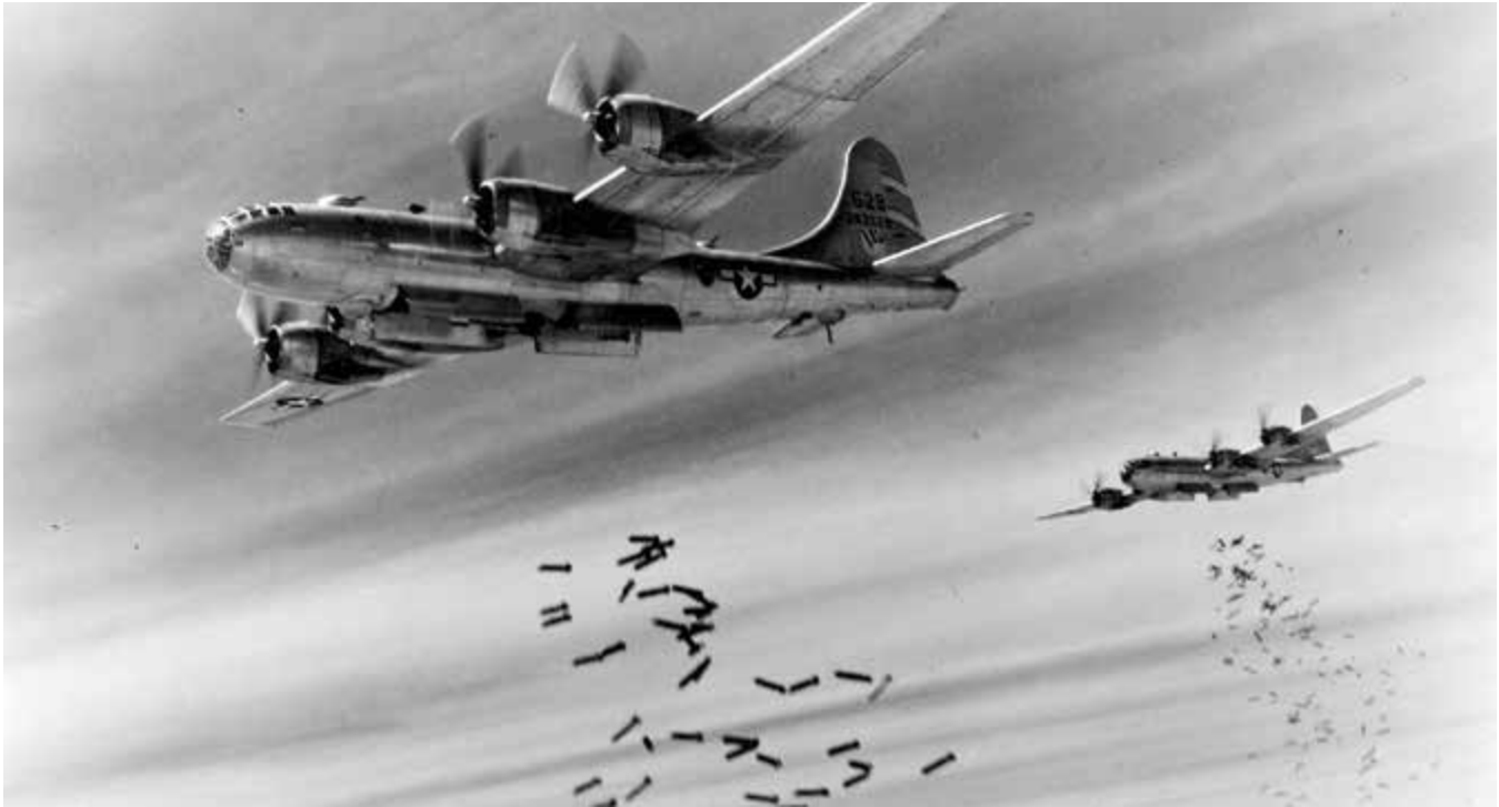
The B-29 was a leap forward in technology and capability. Its cruising speed of 230 mph was 50 mph faster than the B-17 and 15 mph faster than the B-24. (Air Force/Flickr)
