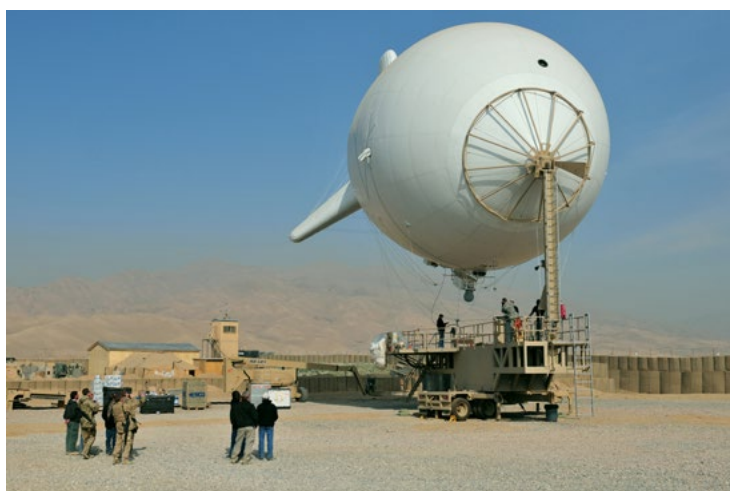
A persistent observation system (aerostat), equipped with high-resolution cameras and high quality live-streaming video monitors, is prepped for deployment at a U.S. forward operating base in Afghanistan in December 2010. Aerostat systems would be a component of the border security system between Jordan and a future Palestinian state. (Chief Petty Officer Matthew J. Thomas/U.S. Navy)
