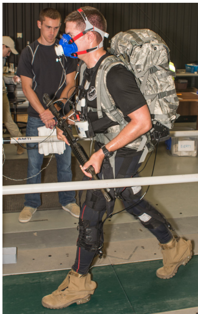
A soldier walks on a treadmill wearing an exosuit developed through the Warrior Web program while researchers at the U.S. Army Research Laboratory measure the soldier's energy expenditure. (Ron Carty/U.S. Army)
