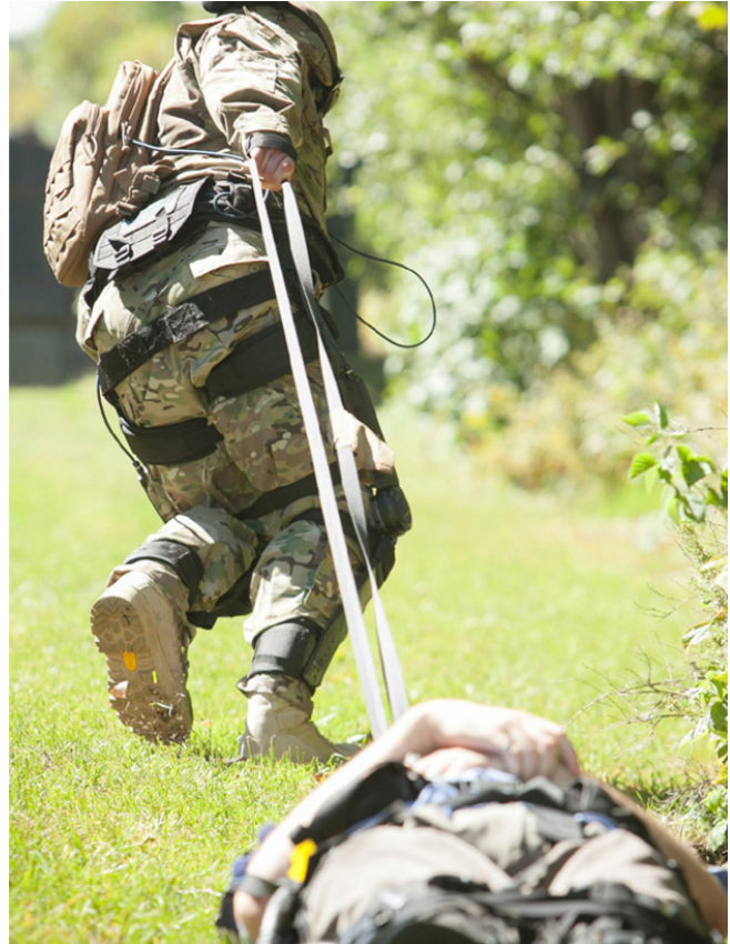
A soldier demonstrates the Lockheed Martin ONYX lower body exoskeleton. Exoskeletons can assist warfighters in carrying heavy loads over uneven terrain with reduced energy expenditure, allowing greater mobility, reduced fatigue, and improved mission performance. (Lockheed Martin)
