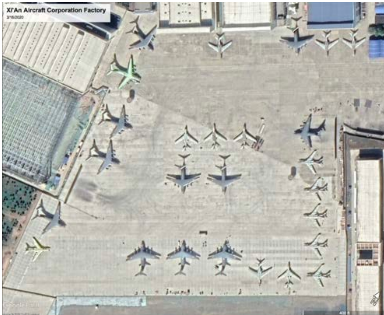
Figure 4: New H-6 bombers and strategic airlift aircraft under construction in Xi'an, China, March 2020. Source: Google Earth.
