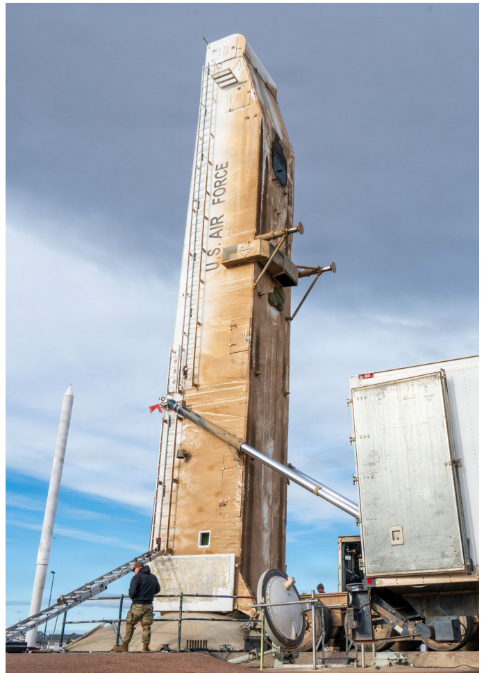
A U.S. Air Force Payload Transporter Erector is placed over a missile silo trainer at Malmstrom Air Force Base, Montana, March 20, 2026. (Photo by Airman 1st Class Ethan Wilson / U.S. Air Force)
