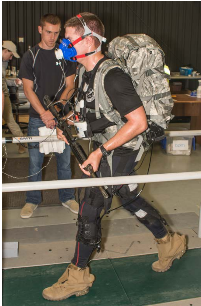
A soldier walks on a treadmill wearing an exosuit developed through the Warrior Web program while researchers at the U.S. Army Research Laboratory measure the soldier's energy expenditure. Exosuits could yield gains of 15 to 20 percent in reducing soldiers' energy expenditure while moving. (Source: Ron Carty/ U.S. Army)
