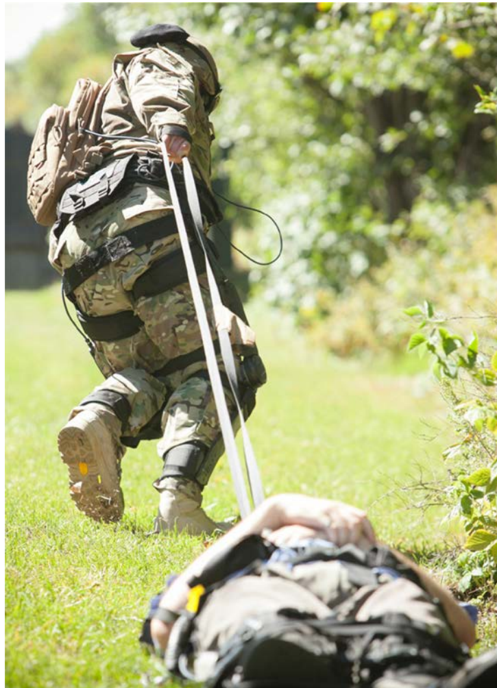
A soldier demonstrates the Lockheed Martin ONYX lower body exoskeleton. Exoskeletons can assist warfighters in carrying heavy loads over uneven terrain with reduced energy expenditure, allowing greater mobility, reduced fatigue, and improved mission performance. (Source: Lockheed Martin)
