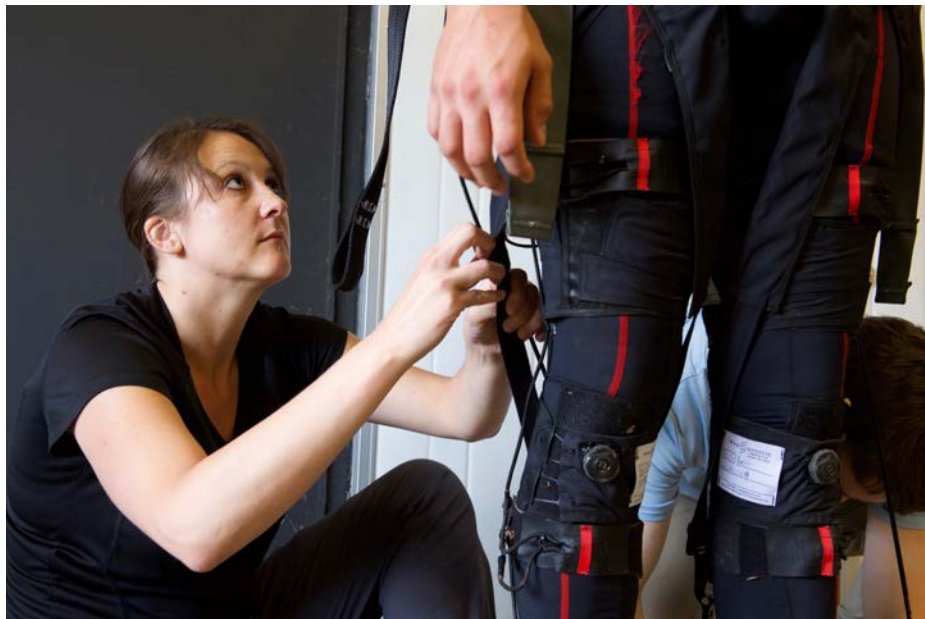
Dr. Courtney Webster adjusts the fit of a soft exosuit developed at Harvard's Wyss Institute through the DARPA Warrior Web program. Soft exosuits augment movement, acting as artificial muscles and tendons, but are not load-bearing like exoskeletons. (Source: David McNally/ Army Research Laboratory)
