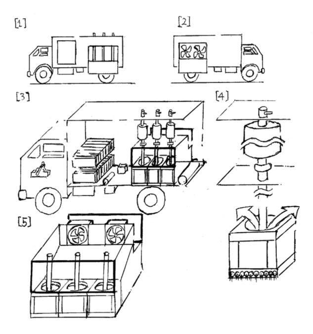
refrigerated delivery truck equipped with a vaporizing device consisting of a heater and a fan at the KG building in Kamikuishiki. <sup>178</sup> As indicated by the diagrams in Figure 5, the design of the second truck was considerably more sophisticated.
