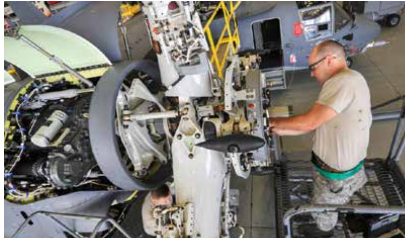
An airman performs maintenance on the engine on a CV-22 Osprey tilt-rotor aircraft at Hurlburt Field, Florida. A high state of readiness will often incur high maintenance costs. (DoD/Flickr)
