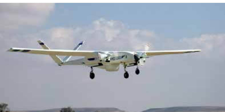
While it looks like a private twin-engine passenger aircraft, the Israeli Hermes 1500 UAV is a twin engine, medium-altitude, long-endurance system. Israel has been a leading exporter of drones. (Israel Defense Forces/Wiki Commons)
