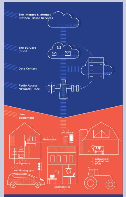
The internet and internet protocolbased (IP-based) services — Internet protocol-based services direct data traffic according to rules called the internet protocol suite, or TCP/IP. Data traffic is divided into small units called packets that are like envelopes; they contain a header, written in internet protocol language that indicates how and where the packet will travel, and the data payload. The internet, one type of IP-based service, is a network of networks that operates on TCP/IP.
