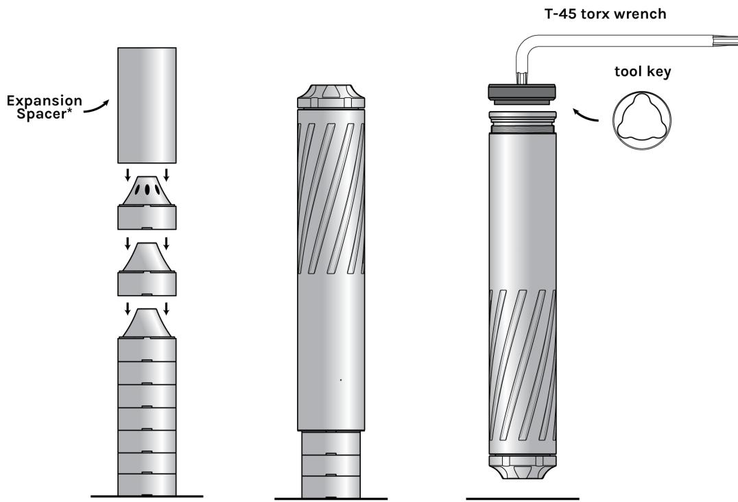
\*As mentioned, the expansion spacer will not come out once the suppressor has been fired. In rare cases, the spacer may dislodge and come out during disassembly. Simply clean and position the spacer on top of the baffles as shown in the illustration above. Continue assembly as instructed.
