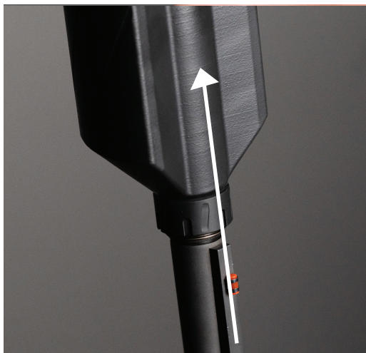
STEP 4 : Align and time the suppressor. Your sight picture should be unobstructed when aiming.
