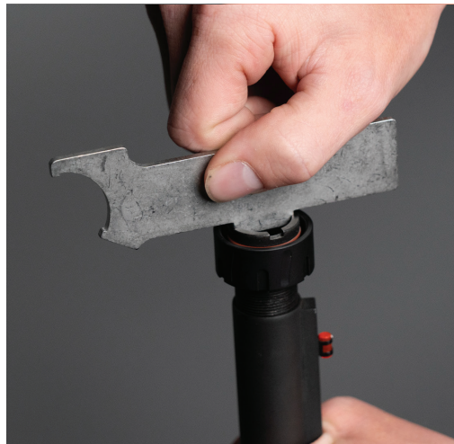
STEP 2 : Thread and tighten choke mount using the takedown wrench or any choke tool.
