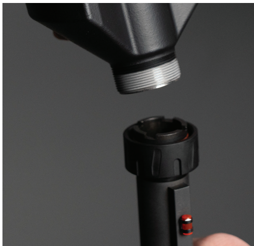
STEP 3 : Attach the suppressor to the choke mount.
