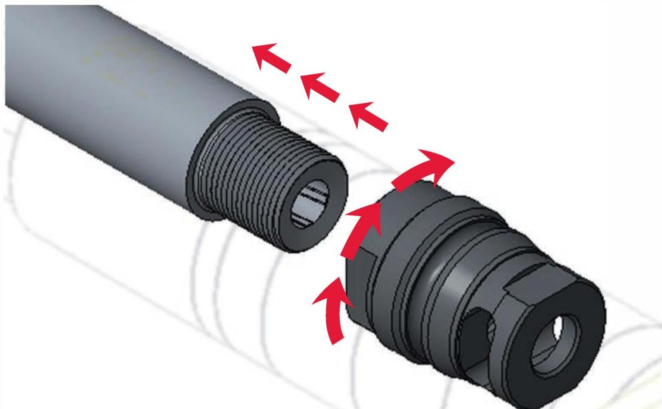
**Note:** If the Regulator mount loosens due to extreme heat cycles, then it's recommended to degrease the threads and use a high temperature threadlocker. LMT AT recommends using a medium strength, high temperature threadlocker like Hot Lock or Rocksett.
