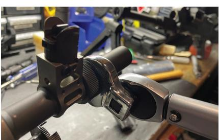
Install the muzzle device (V762MG1FHL) to barrel and torque to 40 ft/lb. No shims are required and there is no specific timing needed. Allow 24 hours for thread locker to cure.
