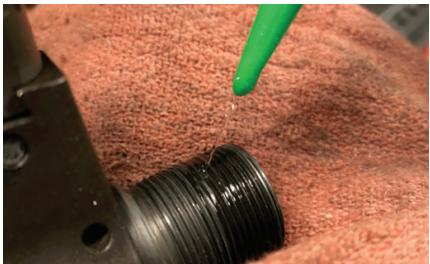
With a standard solvent, such as acetone or MEK, clean the barrel threads using a brush and rag. Allow solvent to dry and repeat process as necessary until any oil is removed.
