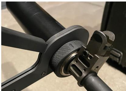
Utilize the locking wrench over the wrench flats to engage the suppressor. This will ensure positive retention when hot and aide in breaking any “locking” experienced from excessive use.
