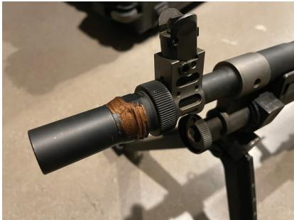
it is recommended to evenly apply a high-temp copper anti-seize to external threads and the gas seal taper of the muzzle device. Ensure device is clean and free of oil and debris.
