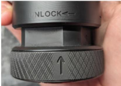
Rotate the locking collar to the UNLOCK position as indicated by the arrow direction and its final position pointed at the tip of the suppressor body arrow.
