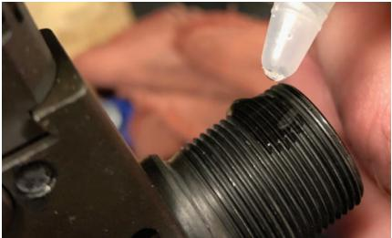
It is recommended to apply a small amount of thread locker such as Rocksett to the barrel threads. This will aide in ensuring the muzzle device will remain in place under extreme duty.
