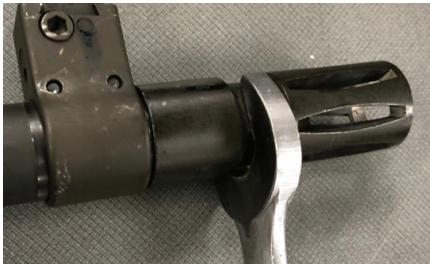
Utilizing available wrench for servicing weapon, remove existing muzzle device. Ensure barrel threads are not damaged in removal.
