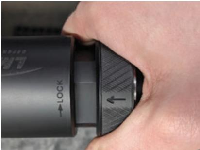
Rotate the locking collar by hand. Locking pawls will engage teeth with a felt and audible “click” into their fully engaged position.
