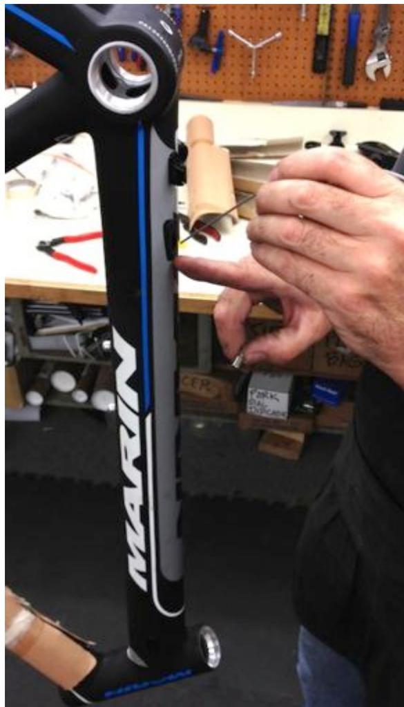
2. Insert a length of cable into the upper frame port and slide down near the lower opening. Use the magnet to help locate the cable through the carbon tube. The magnet will work on steel or stainless cables, as there is usually enough ferrous material in stainless cables to be magnetized. If you do have trouble with a stainless cable however, you can substitute with a thicker gauge brake cable. To protect frame finishes you can also apply a piece of tape over the magnet.
