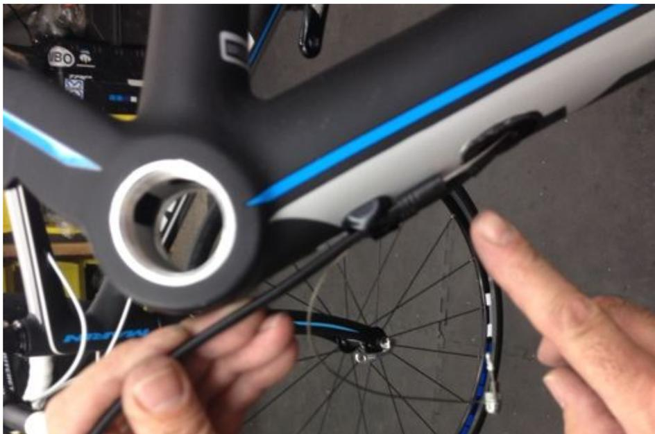
2. With the cable still running through the downtube, slide the plastic over the cable and slide the sleeve up through the frame.
