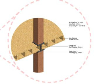
Wood and steel as a modular platform, easily added and detatched matching the society requirement in an irregular leftover space.
