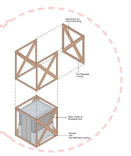
experiment in wood material as a sustainable material, as a core part of a tower structural system. This wooden core is easy to be added on upwards vertically following the modular building organic arrangement
