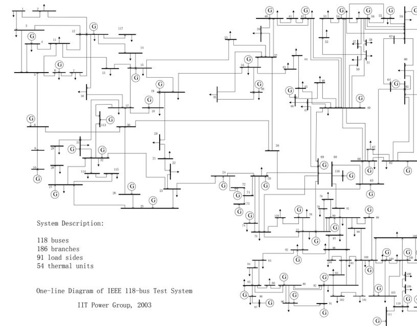
Illustrative One-Line Diagram of the IEEE-118 Node Test Case [3]
