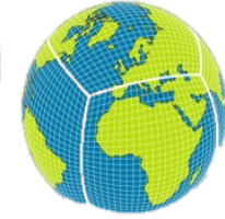
Cubed Sphere Grid e.g., LFRic (Met Office), GFDL FV3
