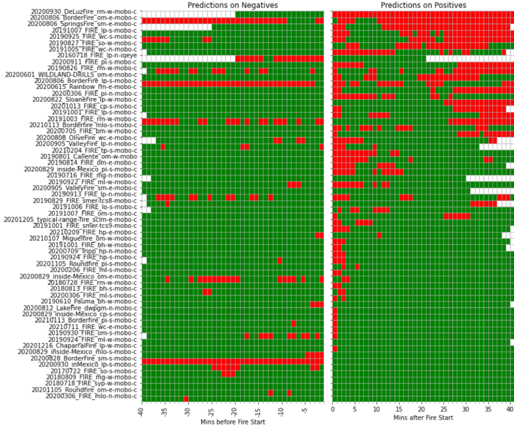
Figure 2: SmokeyNet’s performance per fire on both negative and positive images. Green denotes a correct prediction; red denotes an incorrect prediction; white denotes images missing from the sequence. Common false negatives include faint smoke occurring at the start of the fire or dissipating smoke at the end of the fire sequence. Common false positives include low-altitude clouds and haze.
