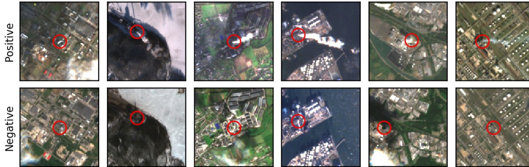
Example images from our image data set. Each column corresponds to a different location; the top row shows locations when a smoke plume is present (positive class), the bottom row shows the same locations during the absence of smoke (negative class). Red circles indicate the approximate origin of the plume.
