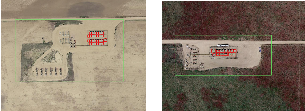
Figure 2: Individual well pad detections. Red boxes are on-pad storage tank detections
