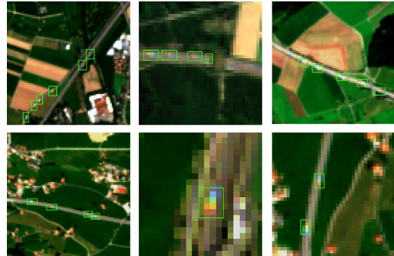
Figure 1. Observations of moving CVs (green boxes) in Sentinel-2 satellite imagery. The “rainbow”-effect is caused by a temporal delay between acquiring the individual bands.
