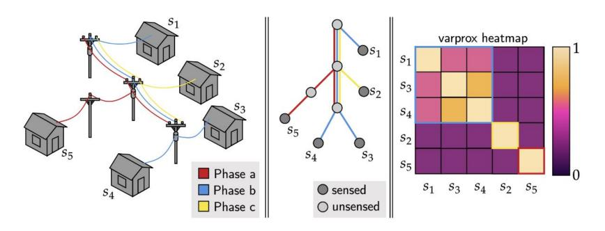
An example network topology (left) and corresponding algorithm result (right)
